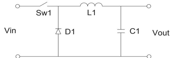
MPS Industries designs these inductors with a wide range of core materials and construction methods based on cost, performance, and size considerations. Inductors have an inherent DC resistance (DCR) which impacts the performance of the output stage. This could also be changed or minimized by winding with different wire types such as magnet wire, litz wire, or Helical edge wound flat wire.
